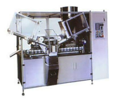
The SD-QRGF-160 automatic paste filler and capper is a kind of completely automatic filling capper packing machine. This filling sealing machine adopts the most advanced pneumatic and electron machinery motion principle in China. The equipment is full automatically that can finish the whole processes of auto-dropping, pipes filling, no filling without pipes, electron scanning, and sealing together.
