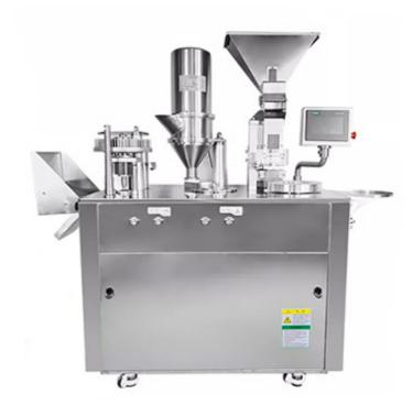
The improved capsule filling machine CGN208-D1 is simpler to operate with less maintenance and better filling quality. The new capsule seeding, filling and locking system increases productivity and lengthen the machine uptime. It is designed for mid-volume customers to provide up to 18 months of uptime without preventative maintenance.
