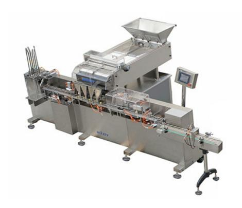
The materials feeding into box from top side. Can be connected with electronic tablets counting machine, weighing machine, carton sealing machine as a production line for the quantitative products.
