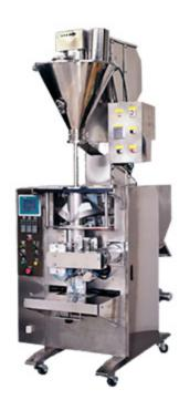
Suited for filling food, pharmaceutical chemicals, and agricultural chemicals. 35 - 65 angle of repose or particle allowed break, and other non-free flowing powders.
