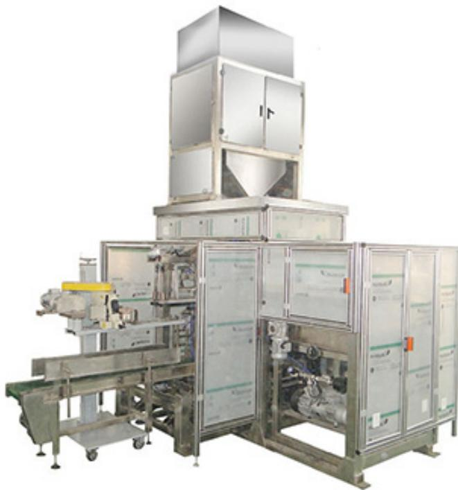
ZTCK-25 Automatic Bag Feeding Packing machine unit is specially suitable for powdery material, the packaging material is paper bag, PE bag, woven bag, the packing range is 10-50kg, the maximum speed can reach 3-8bags/min. High efficiency, advanced design suitable for various requirements.
