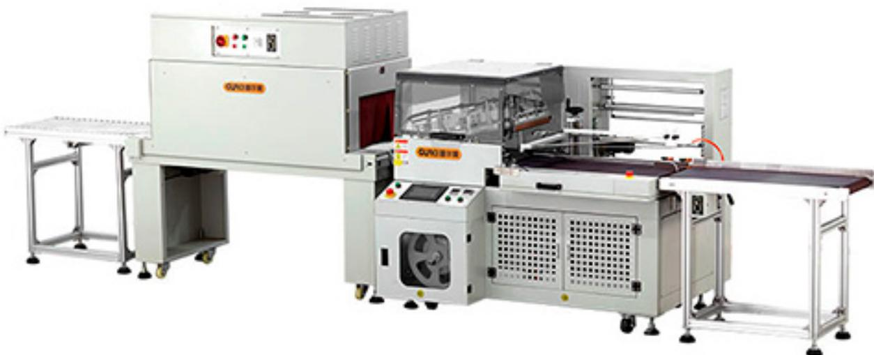
Auto L-Bar Shrink Wrapping Machine is widely used in packaging requirement for batch production, high efficiency, auto film feeding and punching, auto film wrapping, sealing and cutting, manual adjust film guiding system and in-feeding conveyor for different width and height products.
