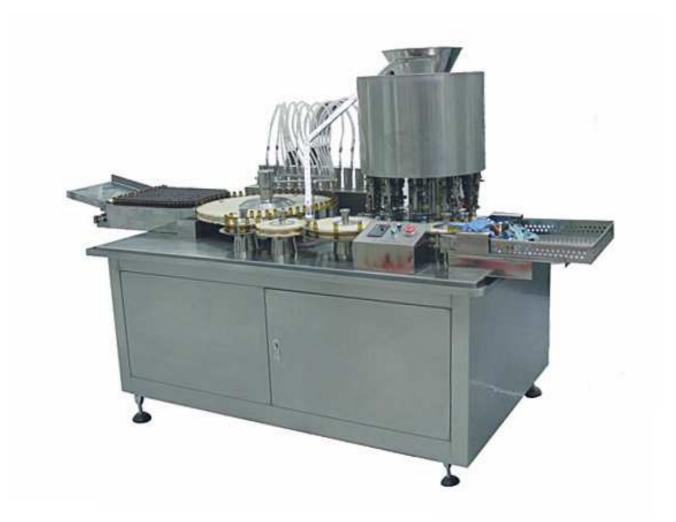
This machine is the main filling & sealing equipment of the oral liquor production line, which is mainly applied in the filling and sealing of 5-10 ml or 20 ml bottles.
