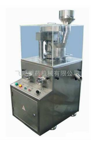
ZP7D Rotary tablet press is a new generation product by our factory, and this machine is a single roller continuous automatic tablet press for pressing various kinds of different shape tablets and plain tablets, such as round tablet, irregular tablet and carved tablet etc.
