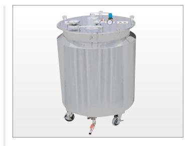
The (Liquid) solution is contained in this tank and transferred to the spray guns. The low height design is aimed at easy maintenance. The compressed air driven motor is adapted for the explosionproof environment. (Film coating: Single-jacketed / Sugar coating : Double-jacketed)
