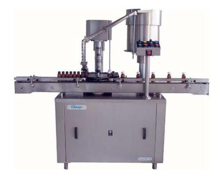
"GMP" Automatic Screw Capping Machine is versatile, self-supported on stainless steel leg with height adjustable adjustment system. The machine is precision built on sturdy welded steel frame completely enclose in stainless steel sheet and doors are providing to facilitate the servicing of machine.
