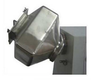
The Octagonal Blender is a based on a movement, which through its tumbling effect produces in the shortest possible time a homogeneous mixture. The product to be mixed is treated very gently. This apparatus can be mounting on Main Drive the housing is manufactured from stainless steel. This Attachment is Suitable to Attached in our All Main Drives
