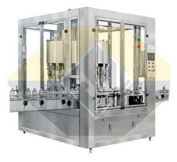
VFO-20XM Automatic 20 Heads Rotary (Piston) Oil Filling Machine is new-generation quantitative filler, with spermatic productivity and high automation. It widely apply to foodstuff, pharmacy cosmetic and chemical, pesticide. The filling volumes range is 50ml-1000ml, the max filling speed can reach 12000 bottles/hour.
