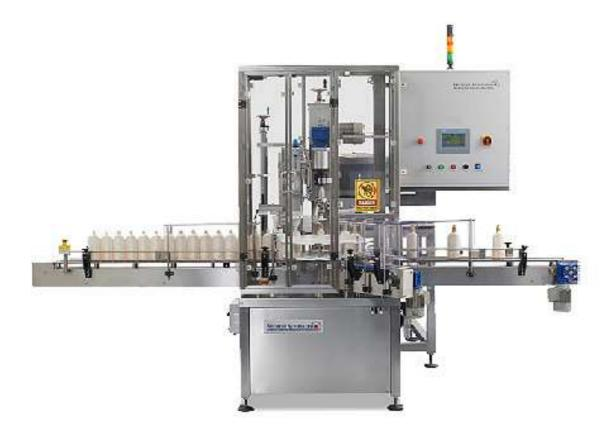
The Alantra series is a fully automatic, versatile automatic trigger and spray pumps capping machine, suited for a variety of containers.
