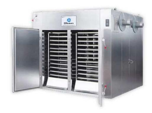
The series of products completely adopt axial fan equipped with automatic constant temperature control system, which is provided with computer control system for option. The working principle is to make use of the steam or electric heat source, through heating the air by heat exchanger and adopting the axial fan as the driving power, the moisture content of hot materials is reduced so as to realize the purpose of drying.
