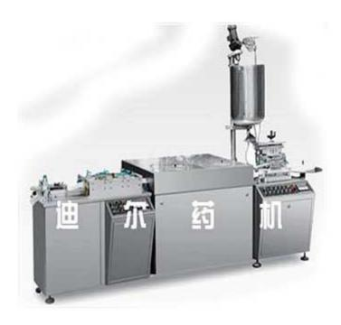
Description: This machine which is manufactured by our company in the latest is mechatronics new equipment for producing suppository. It can finish filling automatically, take shape hypothermia, repair form, seal and shear mono plate.
