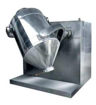
This machine is suitable for mixing dry powder material of pharmaceutical, chemical and food industries. It is used in mixing evenly and quickly between different proportion and fineness of materials.
