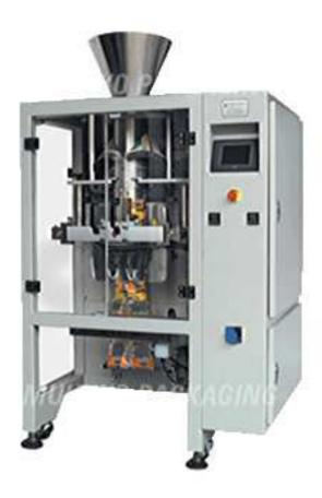
The MK-504 is a High speed servo driven vertical form, fill and seal packaging machine designed to package various powdered products. This servo driven VFFS packaging machine is equipped with servo drive and it uses screw type servo driven auger dosing system to produce center sealed pouches also commonly known as pillow pack or fin seal type pouches / bags.
