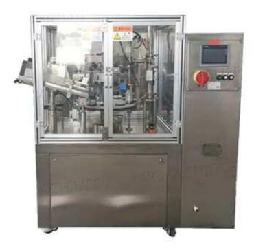
An aluminum tube filling and sealing machine is mainly used for aluminum tube filling and sealing.
