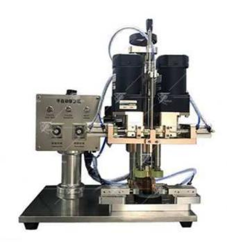
This machine is a fully automatic cap screwing machine. It is widely used for bottles with pump, duck-billed cap or round cap, etc
