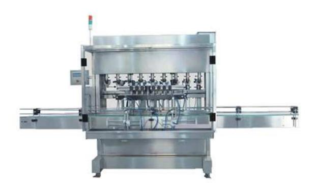
This pneumatic filling machine is apply to filling different fluid, and adopt pneumatic piston to raise the pressure. Measuring by the volume, the switch controls the piston pushing route, ensure the accurate measuring.
