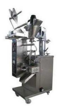
The machine is designed and manufactured specially for powdery and super fine powdery products Driven by servomotor, the auger is rotating to fill products; furthermore, the filling range can be adjusted automatically through computer The processes of bag making, measuring, filling, sealing, cutting, counting and hot pressing codes can be done automatically. Packing material include several kinds of heat-seal lamination, such as PET/plated AL/PE, PET/PE, NYLON etc.
