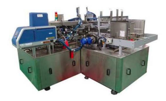
GB series includes automatic machines for the packaging of pvc bottle, pet bottle, glass bottle, paper and box in corrugated cardboard cases and/or trays without film which widely used in food, toy, chemical, cosmetic, medical and plastic industries. Wrap around case packers can achieve an output up to 35 packs per minute, according to the product. The packing arrangement can vary according to the containers shape and dimensions; in general, the most requested arrangement are: 2x3, 3x4 and 4x6.
