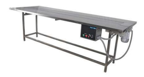
The packing conveyor belt is having stainless steel table top with moving endless sandwich belt in the center. Tabletop is fixed to the same structure made out of SS square pipe & supported on adjustable bolts. Tabletop is of 12 inches working space on both side of the conveyor belt for final visual inspection & packing into the box.
