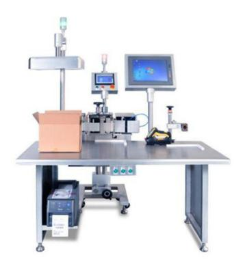
HYCP-200 enables real time printing and application of labels on to product packages. Information such as production data, serial & batch numbers, anti-counterfeit numbers, unique product ID, packaging data, and distribution channel data etc. can be printed to the label in characters, barcodes, or 2D codes, or even in the form of RFID. Automatic application of these information on-line enables effective track and trace of the products.
