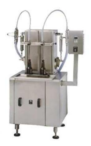
**Filling Range:** 5 ml to 1 Liters (With the help of Change Parts) **Output:** 12 to 15 bottles per minute for 1 Liter. (Depending upon Liquid and Bottle)
