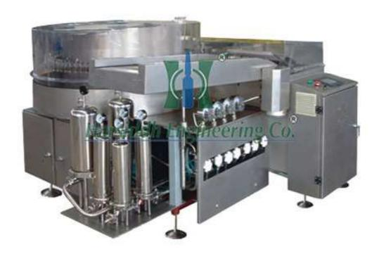
Harsiddh rotary ampoule washing machine is a state of the art device that is designed to aseptically clean ampoules with minimum contact between the machine parts and the container. The equipment has a specially designed automatic gripping mechanism that holds ampoules from the neck, inverts them and cleans them before discharging them in the feed worm system at upright position.
