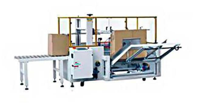
The automatic case erector opens, forms, and fold cartons, sealing with tape or glue as needed before sending the empty carton to the packing machines. This high speed case opening machine can prepare large quantities of cartons at a time and is easy to operate with a PLC and touch screen.
