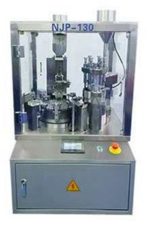
NJP-130 adopt PLC control system, human-machine interface, when running malfunction or lack of stuff, automatic alarm, malfunction display, automatic dismiss alarm. And with functions of password setup, touching screen display, automatic parameter setup, data printing, reset, etc.
