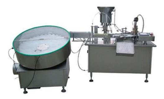
This machine is specially designed for filling and sealing plastic bottles that are easily broken, and its working procedures include automatic bottle feeding by unscrambler, bottom filling, automatic capping, sealing, and the like.
