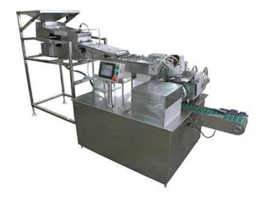
JZJ-40 tablet rolling paper machine is a packaging machine that rolls a sheet of paper or aluminum poise paper into a roll of certain amount.
