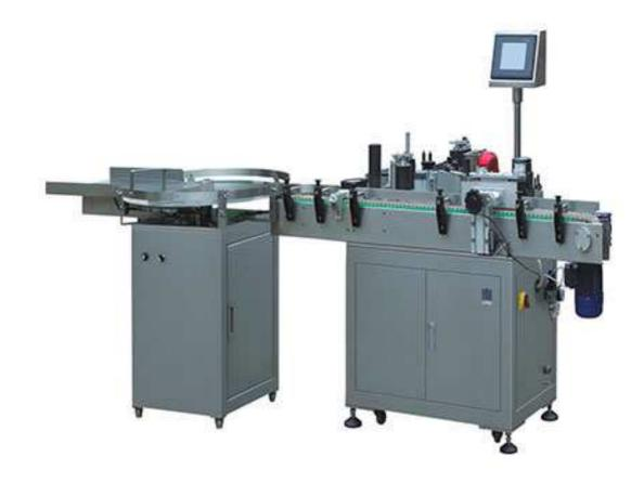
Automatic labeling machine for the application of labels on round bottle. The machine is composed by a conveyor, one of label adaptor and one of label applicator. In case of wrap around label application a side conveyor is installed. There is also the possibility to install a hot stamping unit, print expiry date, batch code etc. The bottle loading/unloading can be done manually, through loading/unloading turntable (alternative Ø620mm or Ø900mm) or directly from an production line.
