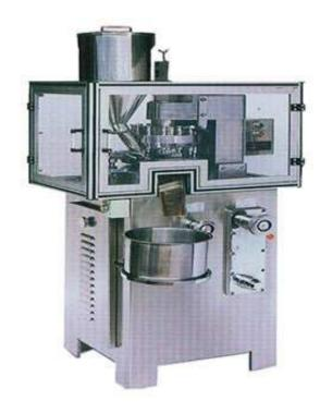
The rotary table machines are used in various branches of the industry for the tableting of the powders. They are used in the chemical and pharmaceutical industry and also in the industry for plastic materials. In the industry for plastic materials the rotary tablet machine is used for preforming the raw material by means of a cold working because it give to the same material a good consistence. Using the rotary tablet machine there are following advantages.
