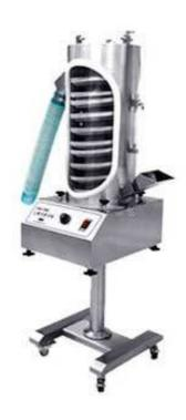
SZS200 Uphill Tablet De-duster is a special equipment to wipe out burr and dust of tablet whilst going up way. It can be connected with tablet press and metal detection systems. 316L stainless steel are used for all metal parts contacting tablets. Design of GMP.
