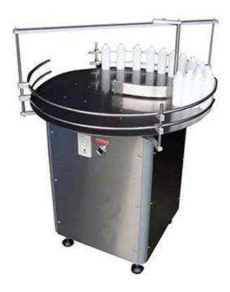
This bottle turntable is suitable for feeding or collecting "Round Bottles" automatically in a production line. Much production efficiency can be improved and labor cost will be lowered while not feeding and collecting bottles manually.
