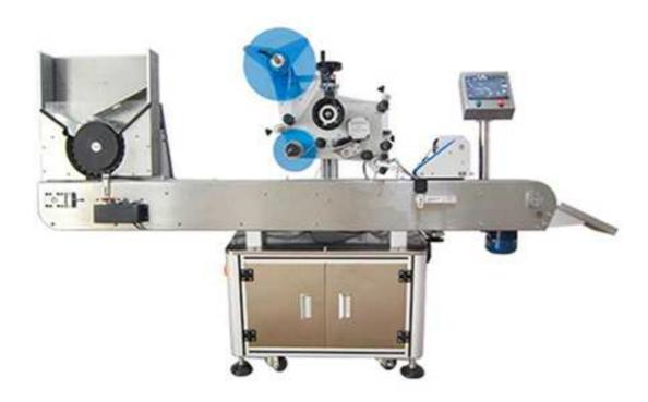
The Horizontal Wrap-Around Automatic Labeling machine has few moving parts, and adjustments are easily made. Changeovers are easy by simply swapping out the container.
