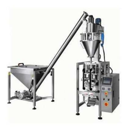
The powder filling machine is a powder filling machine, which is suitable for quantitative filling of powdery and granular materials such as pesticides, veterinary drugs, premixes, additives, milk powder, starch, condiments, enzyme preparations, and feeds.
