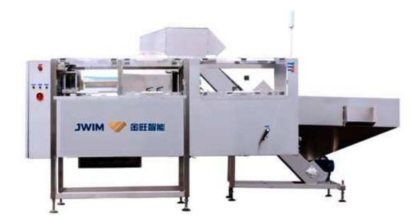
Automatic Bottle Unscrambler is making up with the bottle elevator, unscrambling rotary plate, bottle rejecting devices, unscrambling and electrical control cabinet. It can arrange the disordered empty plastic bottles into good order. The machine is with the features of compact structure, simple operation, mature technology and stable running and operation.
