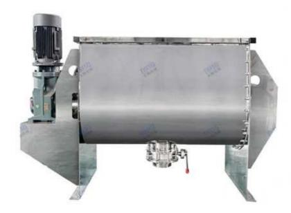
Industrial Ribbon mixer adopts U-shaped cylinder, with a unique structure of inner and outer ribbon, Outer spiral conveys the material move from the two sides to the center and the inner screw conveys the material move from the center to the sides to get a high effective convective mixing.
