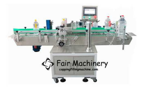
For the pharmaceutical, food, cosmetic and other industries round bottle labeling, can be affixed to the week and semicircular labeling. Optional automatic turntable Unscramble can be directly connected to the front end production line, automatic feeding bottle into the labeling machine, increasing efficiency. Optional configurations ribbon coding labeling machines, online print production date and batch number, reduce bottle packaging processes, improve production efficiency.
