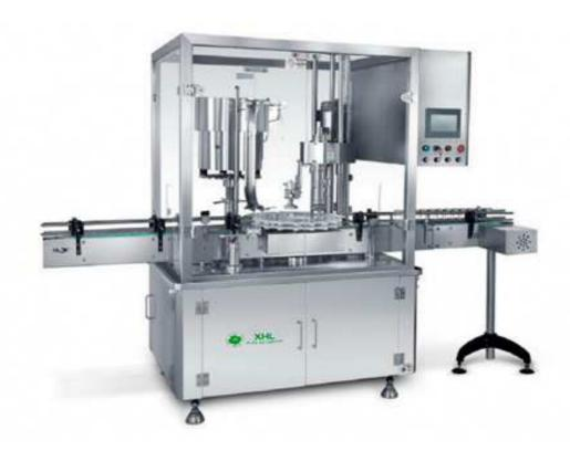
Automatic Economical Round Disc Positioning Type Cap Turning Machine
