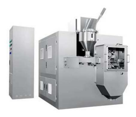
Dry granulation is widely used in pharmaceutical, food, chemical and other industries. It is especially suitable for granulation of drugs that are easily decomposed by moisture, easy to absorb moisture, sensitive to heat, and the particles can be used for densification to improve fluidity, tablet compression, Filling capsules and granules for bagging. Based on many advantages, it is widely used in various industries.
