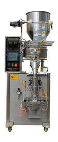
This Automatic Sachet/pouch Packing Machine can put hundreds of bags in the bag-receiving part of the equipment at one time.
