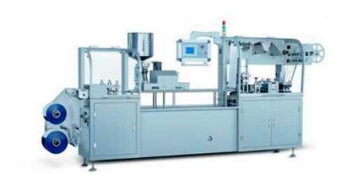
This machine adopts intelligent driver and PLC Human Computer Interface. Strokes can be adjustable with servo motor driver control. The frequency and temperature can be adjusted. The base temperature is 165 degrees centigrade. This machine has pre alarm function for AL-PVC foil end, and alarm light, green color for working state and red color for AL-PVC foil end, in case of opened safety cover and when minimum air pressure is not sufficient.
