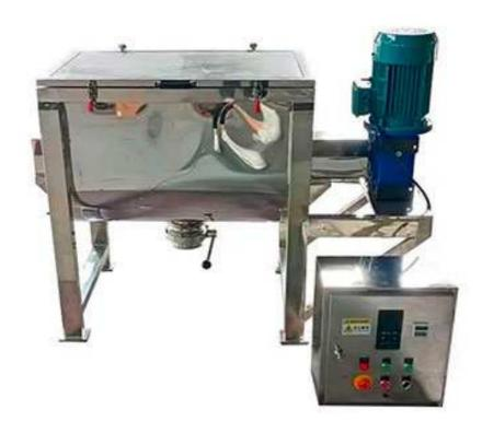
The horizontal ribbon Mixer Machine is made of stainless steel 304 or stainless steel 316 as required. The Mixing Machine is composed of U-shaped container, spiral band mixing blade and transmission parts. The outer spiral belt coiling form in the mixing container matches the rotation direction to push the materials from both ends to the middle, while the inner spiral belt pushes the materials from the middle to both ends, forming convection mixing, so that the materials can be mixed.
