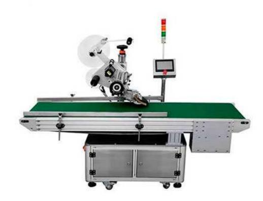
ZF-TBP150 is suitable for labeling on the surface of flat packaging, labeling on the surface of flat packaging for a single roll of tape, and flat labeling on the carton and so on.
