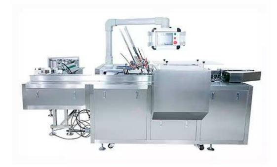
This machine is suitable for packing AL/PL Blister, bottle, Pillow Type Bags and other related similar content compact automatic leaflet folding, box opening and loading, batch number embossing as well as sealing technology processes. (Options hot-glue device extra)
