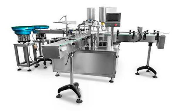
The CapperPacks Automatic Capping Machine is suitable for automatic capping and screw capping of bottles. The bottle feeding and conveying can be connected from last process, and the bottle can also be placed manually, and the cap is automatically vibrated to send and screw the cap.
