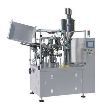
The ZHF-80Z laminated tube filling sealing machine is always applied to pack ointment and paste. Beyond that, it can also package cream, gel and sticky liquids. Presently, our ointment filling machine wins wide application in cosmetics, foodstuff, pharmaceutical and light industry. Generally, ZHF-80Z adopts twice folding, triple folding and saddle tube tail folding.
