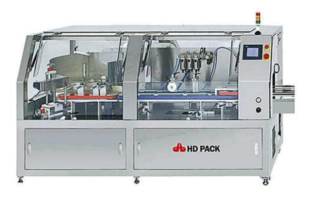
Once bottles are poured into unscrambler hopper, bottles are conveyed by escalator to the turn table. Randomly arranged bottles are being arranged in order by centrifugal force in turn table and sufficient numbers of bottle are always remained in turn table by sensor detection. Hooker in the machine arranges bottles in one direction which are conveyed by side belts conveyor, then reverse bottles.
