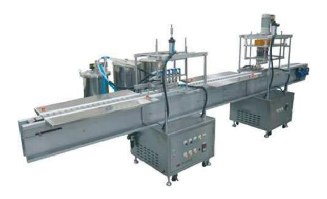
manual put empty bottles on conveyor→auto filling→manual feed cap→auto locate the cap→auto capping→manual collect product
